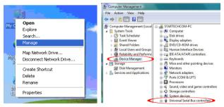
In the Device Manager, under the Universal Serial Bus Controllers category, you should see the new entries for the USB 3.0 controller card.
