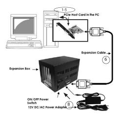
1. Turn OFF the computer power before installation, and remove the chassis cover from the computer. Similarly, ensure the PEX2PCI4 is not powered at this time.
