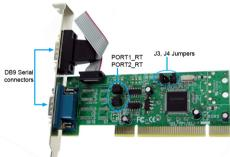
The two sets of jumpers on this card (J4, J3 and PORT1\_RT, PORT2\_RT) are used to configure the operating mode/serial protocol and 2/4-wire operation respectively.
