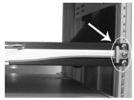
3. Slide the assembled drawer into the rack cabinet from the front and insert the two slide rails of the assembled drawer into the pockets of the rear brackets.
