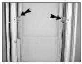
Remove the safety stopper from the console drawer. The safety stopper is designed to prevent the drawer from sliding out during transportation. Please note that once the Safety Stopper is removed, the drawer is free to slide out when the console is tilted. Be cautious, as this could cause injury.
