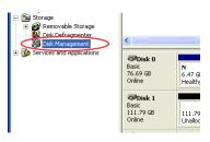
Locate the Disk that says it is "Unallocated" (check hard drive capacity to confirm it's the correct hard drive) and then right-click in the section that says "Unallocated" and select "New Partition".
