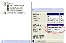
If you are installing a hard drive that already has data on it, then after plugging it in, the drive should automatically show up with a drive letter assigned within "My Computer". You can verify or change the drive letter through Disk Management, as outlined above.
