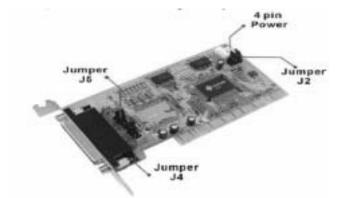
The card uses jumpers to set internal and external power voltages, and to configure which serial ports will receive 5v, 12v, or RI signal (unpowered) through the 9th pin.
