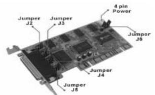
The card uses jumpers to set internal and external power voltages, and to configure which serial ports will receive 5v, 12v, or RI signal (unpowered) through the 9th pin.
