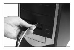
3. Continue to feed the cables into the computer case (through the open drive bay), until the ExpressCard Bay is near the opening, then press the ExpressCard Bay into the case so that it is flush with the face of the computer case:
