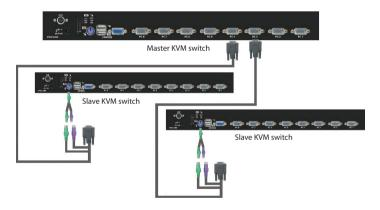
The maximum number of computers controlled by a Master/Slave configuration with all 8-port units is 64, with 8 Slaves and each Slave connecting to 8 computers:
