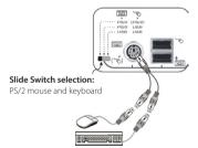
PS/2 Keyboard and USB Mouse: Slide switch to the center position
