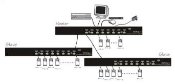
After the connection has been completed, please re-activate the OSD menu to verify that the Master recognizes the Slaves. A triangle mark ( $\blacktriangleright$ ) is placed next to the right of the channel name indicating that the port is connected to a Slave, not a computer. A number to the left of the triangle mark indicates the Slave model, i.e. '8' for an 8-port switch.
