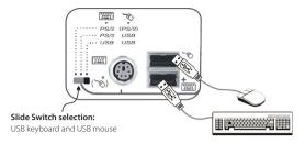
**NOTE:** When configuring the switch as a Slave in a cascaded configuration, PS/2 Keyboard and Mouse is the only mode that can be used. Therefore, SV431DUSB cannot be configured as a slave in a cascaded setup, as it does not provide a slide switch selector.
