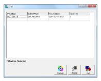
To refresh the status of the adapter network connection, click 'Refresh' on the lower right corner. This shold be performed following any configuration changes.
