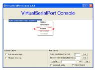
The "Add Net" window will allow you to configure the COM port to the settings used by the NETRS2321E unit you wish to associate with. Select the proper operating mode, network settings used to configure the NETRS2321E unit previously (see Web Console Configuration).
