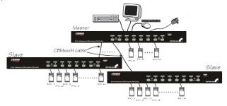
After the connection has been completed, please re-activate the OSD menu to verify that the Master recognizes the Slaves. A triangle mark ( > ) is placed next to the right of the channel name indicating that the port is connected to a Slave, not a computer. A number to the left of the triangle mark indicates the Slave model, i.e. '8' for an 8-port switch.
