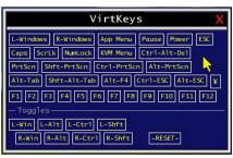
Clicking any button in the top half of the window simulates pressing and releasing the indicated key. In the bottom area of the screen, clicking will simulate the indicated Meta key being pressed. You may then click in the top part to send another key and release the Meta key at the same time.
