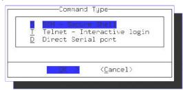
3. If you are choosing "Direct", use the screens that follow to choose the appropriate setting for your serially attached device. If you choose SSH or Telnet, the following screen will ask you for the Host Name or IP address of your remote connection:
