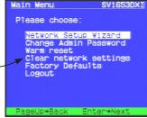
If static IP addresses are assigned, you will likely need to change the Net Mask, IP Address and other details, prior to connecting via your Web browser. If this is the case, connect a local keyboard (USB or PS/2) and press the *Enter* key.
