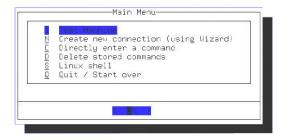
To remove a previously created connection, highlight "Delete stored command" and press enter. You will be prompted for the admin password. Highlight the connection you wish to remove and press enter.
