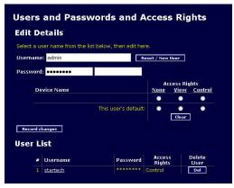
The *Edit Details* section allows you to modify one user account at a time, by clicking on the desired account in the *User List* section. For each host, a user can have:
