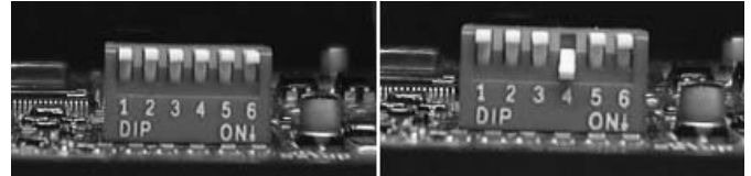
DIP Switch 4 in normal mode ("OFF", "up")
