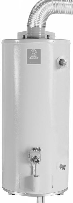
**Direct-Vent Design** - FVIR compliant, one-pipe, dual channel closed-combustion system draws all make-up air from outside the home, eliminating problems caused by insufficient indoor ventilation. Horizontal air intake and venting on all models up to 80 inches from outside wall, with no electrical power needed.
