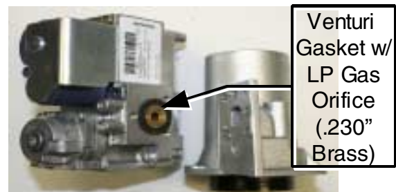
Gas Control with .230" LP Orifice
