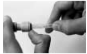
Figure 12 Removing Tubing from fittings
