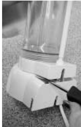
Figure 3 Counter-top stand removal
