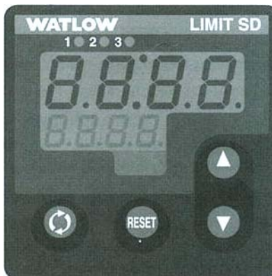
Figure5: Typical Redundant Safety Controller Display
