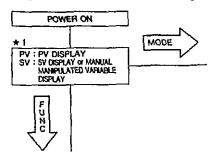
There are two main menus in the MC-125 controller, the Function menu and the Mode menu. These menus are illustrated starting from the top left corner of the Operation Manual (fold out Programming flowchart). The and arrows indicate their direction through the flow chart. The Function menu contains information on the manual tuning of your controller and the Mode menu allows you to turn on the Automatic tuning feature (Autotuning).
