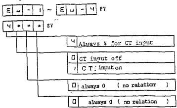
When using the current transformer input for heater break detection, one slot (input) is needed for single phase systems and two slots (inputs) are needed for three phase systems.
