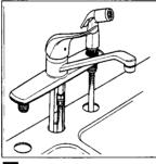
2 Place a bead of plumber's putty around base of faucet. Insert shanks into sink deck holes with spout to front over sink.
