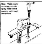
1 Pass spray hose down through hole in escutcheon and extreme right sink deck hole and up through center sink deck hole. Attach spray hose to spray outlet.
