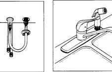
1 Turn on water supplies and check for leaks. With faucet off remove aerator, turn on water rotating hot through cold to flush lines and faucet. Turn faucet off and replace aerator.
