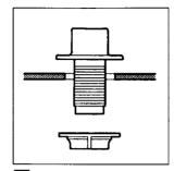
1 If your faucet has a spray, place hole guide down through hole at extreme right of sink top. Add mounting nut to underside and FINGER tighten firmly.
