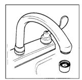
1 Turn on water supplies and check for leaks. With faucet off remove aerator. Turn on hot and cold to flush lines and faucet. Operate spray. Turn off faucet and replace aerator.
