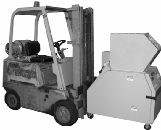
Figure: Lifting the granulator
