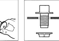
If your faucet has a spray, place hole guide down through hole at extreme right of sink top. Add mounting nut to underside and FINGER tighten firmly.
