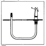
Insert spray hose down through hose guide and up through center hole in sink and putty plate.
