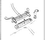
Position putty plate. Apply Teflon tape to spray outlet on body. Attach spray hose to spray outlet by rotating faucet body. Tighten securely with wrench.
