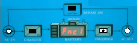
The inverter ins disabled. Only the Bypass switch and charger will work normally.
