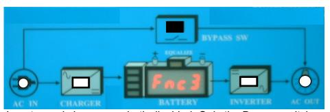
Inverter and charger are both disabled. Only the Bypass switch function is enabled in input and frequency is OK.
