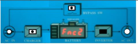
Charger and Bypass switch are disabled. The inverter will work continuously even if there is a correct AC voltage at the input.
