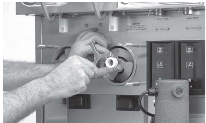
Figure 24. Removing Auger Supports
