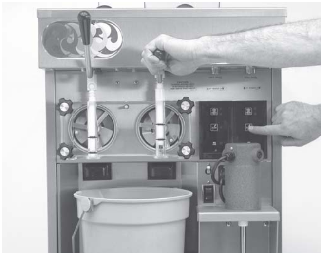
Figure 14. Spigot Opened and Solution Draining
