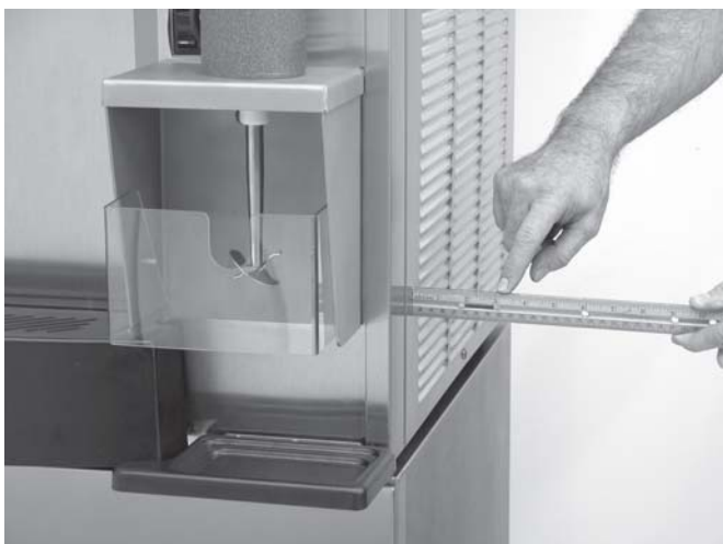
Fig. 4. Space and Ventilation Requirements
