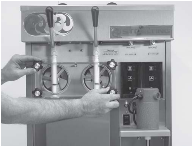
Figure 21. Removing Front Door
