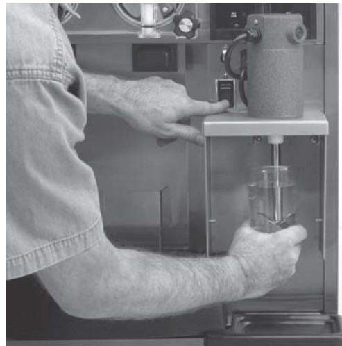
Figure 19. Cleaning Agitator Shaft
