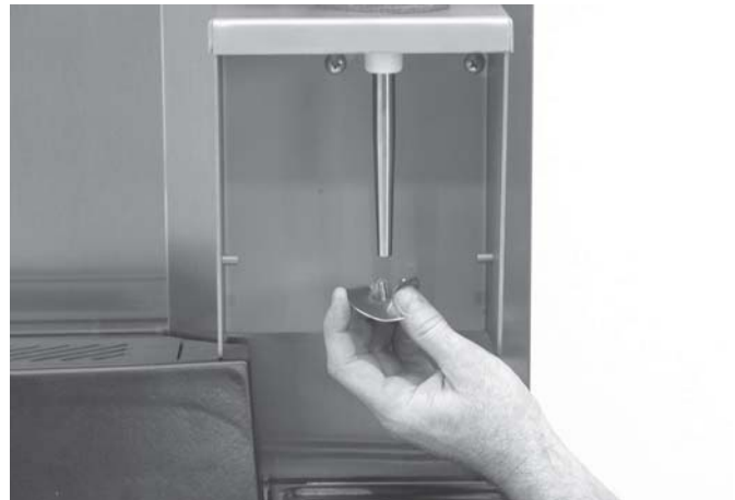
Figure 23. Removing Agitator From Shaft
