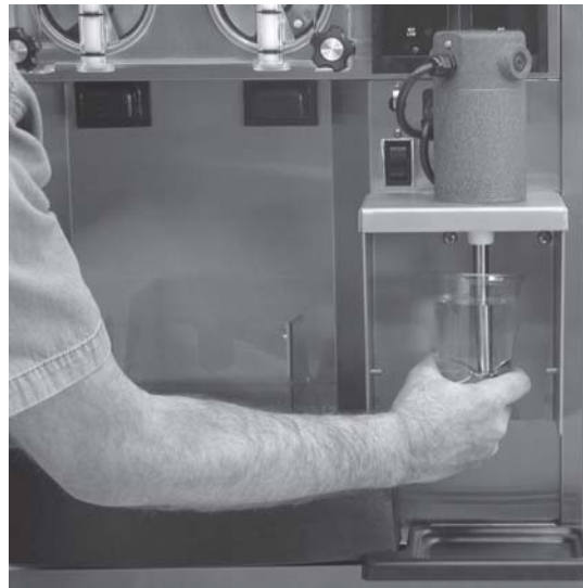
Figure 15. Sanitizing Agitator Shaft
