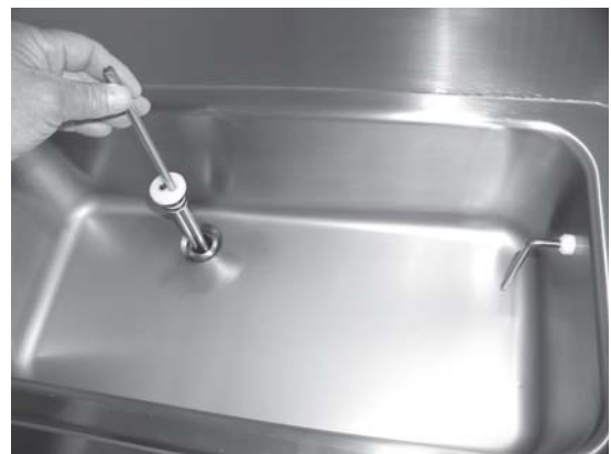
Figure 16. Removing Mix Inlet Regulator
