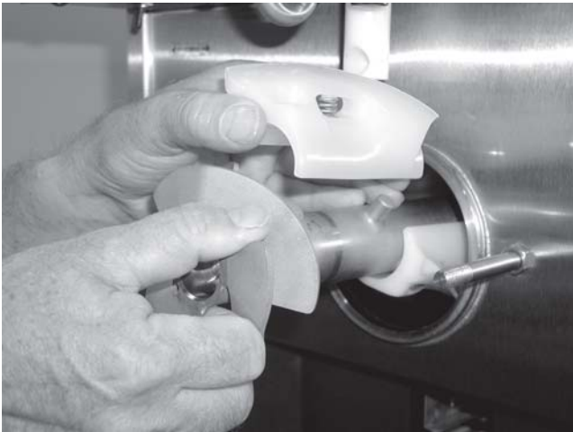
Figure 22. Auger Shaft Removal
