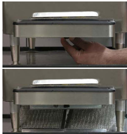
Figure 3-10 E112 Condenser Filter Removal
