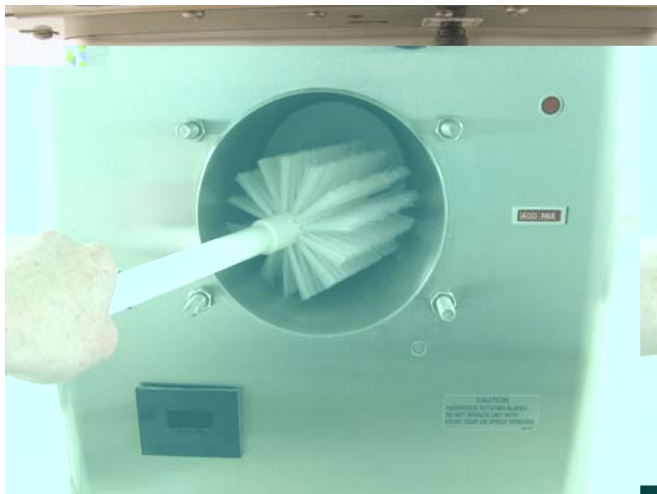
Figure 3-7 Cleaning Freezing Cylinder
