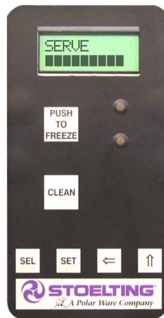
Figure 3-5 During Freezing Cycle
