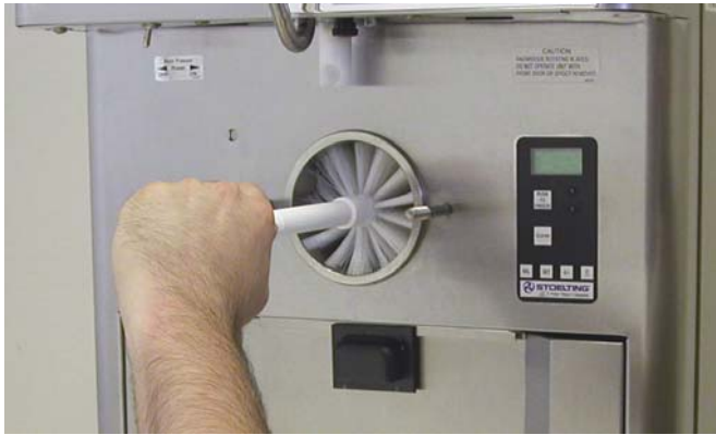
Figure 3-10 Cleaning Freezer Barrel
