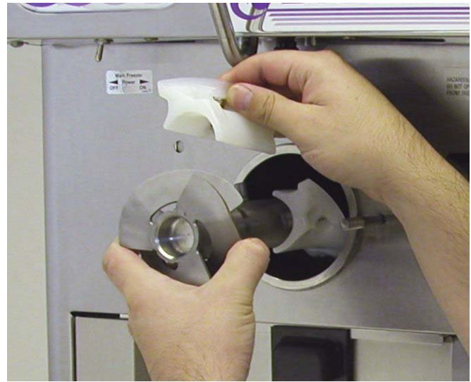
Figure 3-8 Removing Auger Shaft and Flights
