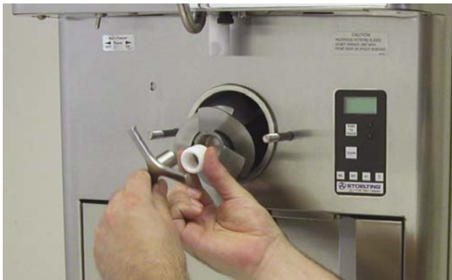
Figure 3-7 Removing Auger Support
