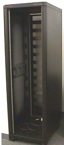
Empty M03 cabinet used for the 9176 controller tray and drive trays
