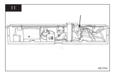
9.5 Reassemble in reverse order and check for gas leaks.
