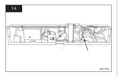
10.6 Remove the feed pipe with the injector attached from the
