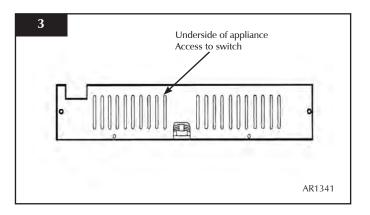
• Use a ball point pen or narrow screwdriver to push the rocker switch to the OFF (O) position, Diagram 4
