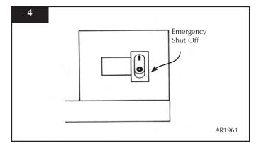
(This switch is set to be ON ( ]) during normal operation and must remain ON)
