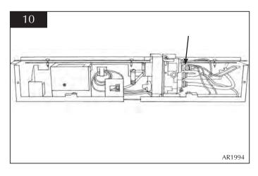
9.4 Support the valve and remove the magnetic valve retaining nut, Diagram 11
