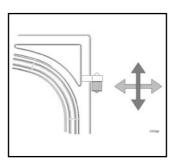
9.3 Using a 20mm A/F spanner loosen the fixing nut inside the stove as shown in diagram 1, and reposition the hinge blocks to achieve a correct fit. This may need a trial and error approach to find the correct position.
