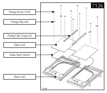
7.3 Using a screwdriver remove the glass clip fixing screws (4). The old glass can then be lifted clear of the door. (Note how the 3mm sealing rope is placed between the glass and the door.) Remember to dispose of the old glass safely.
