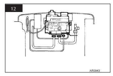
7.3 Reassemble the interrupter block and leads. Secure the thermocouple connection in the rear of the gas control. (Do not overtighten). Turn the gas supply on and check the entire pipework and valve joints for any leaks.
