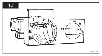
6.4 To release the right-hand side of the control cover, insert the narrow blade screwdriver into the slot shown in diagram 11. Lever it gently and pull from the right-hand side at the same time. The cover will now come off. There is a small cylindrical metal spacer inside the cover. This must be kept and replaced on the fixing screw during re-assembly.
