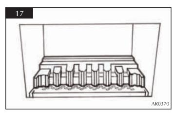
5.15 Locate the front coal moulding in front of the flame baffle ensuring that the end legs sit flat against the burner skin, see diagram 18.
