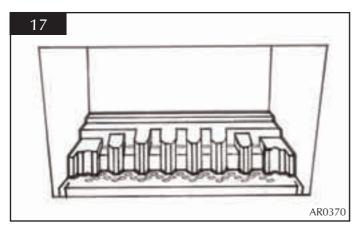
6.15 Locate the front coal moulding in front of the flame baffle ensuring that the end legs sit flat against the burner skin, see diagram 18.
