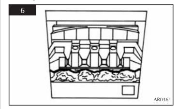
5.4 Place five of the loose round coals on the front coal so that they lean against the flame baffle, in between the fingers. Place the two rectangular coals behind the round coals, one at each side, see diagram 7.
