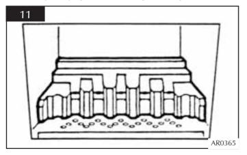
6.9 Locate the front coal moulding in front of the flame baffle ensuring that the end legs sit flat against the burner skin, see diagram 12.
