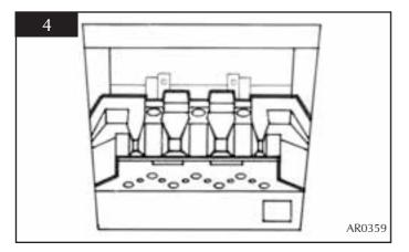
5.2 Locate the rear panel against the spacer brackets and slide down so that it locates on the ledge of the flame baffle, see diagram 5.
