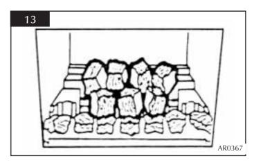
6.11 Place two small coals at each end of the front coal so that they lean against the flame baffle, and a further two large coals on the flame baffle, one at each end, see diagram 14.
