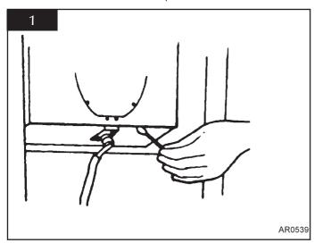
1.2 If there are any extractor fans in adjacent rooms, the test must be repeated with the fans running on maximum and interconnecting doors open.
