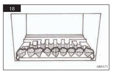
6.16 Place three large coals on the front coal so that they lean against the flame baffle and four large coals on the flame baffle so that they sit on the fingers, see diagram 19.
