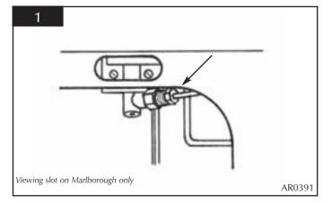
2.2 Disconnect thermocouple from gas valve. See diagram 2. Remove ignition lead from electrode. (Cut cable tie to ignition lead if required).
