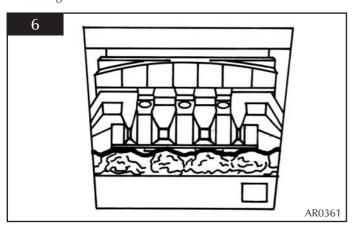
6.4 Place five of the loose round coals on the front coal so that they lean against the flame baffle, in between the fingers. Place the two rectangular coals behind the round coals, one at each side, see diagram 7.
