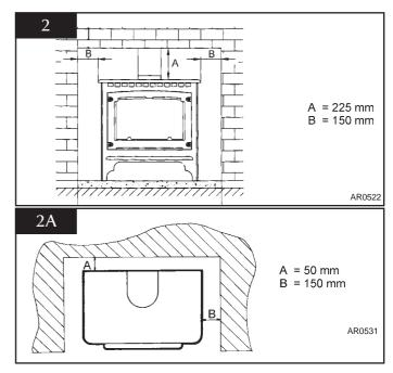
In a non-combustible recess, attention must be given to allowing adequate clearance at the sides and rear of the stove, so that a spillage test can be performed, and the controls reached.
