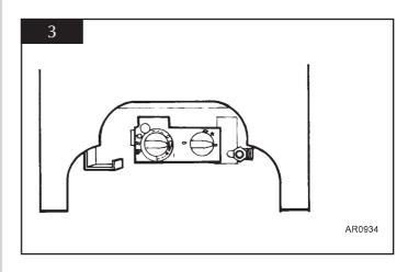
There is a cutout in the RH rear leg to enable a direct straight connection to be made to the rear of the stove. See diagram 3. A gas soundness check must be completed up to the gas inlet connection.
