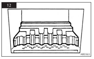
6.9 Locate the front coal moulding in front of the flame baffle ensuring that the end legs sit flat against the burner skin, see diagram 13.
