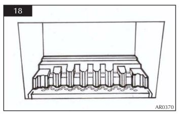
6.15 Locate the front coal moulding in front of the flame baffle ensuring that the end legs sit flat against the burner skin, see diagram 19.
