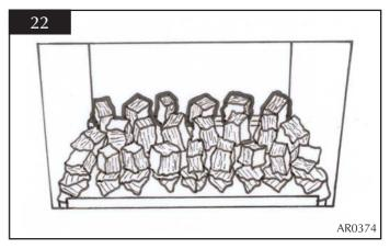
NOTE: ENSURE THAT THE COALS ARE POSITIONED, AS DETAILED ABOVE. ONLY USE THE CORRECT AMOUNT OF COALS, AS SPECIFIED IN DIAGRAMS.
