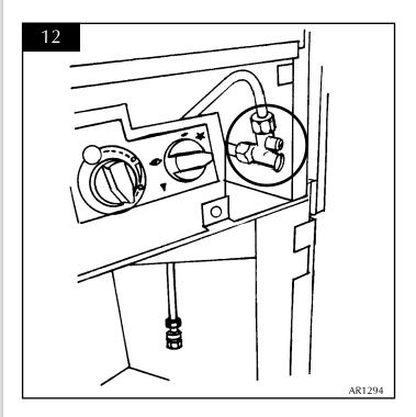
3.20 Light the appliance and check the rest of the joints for leaks. Turn the appliance to maximum and check the supply pressure is as stated on the databadge. Turn the gas off and replace the test point screw, turn the gas back on and check the test point for leaks.
