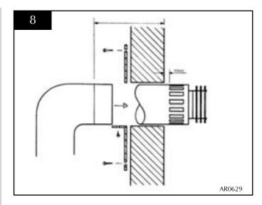
3.14 There is a c ardboard itment in the terminal. This is to support the flue whilst it is cut to length. **REMOVE THE REMAINDER OF THE CARDBOARD AFTER CUTTING TO SIZE**. See diagram 9.
