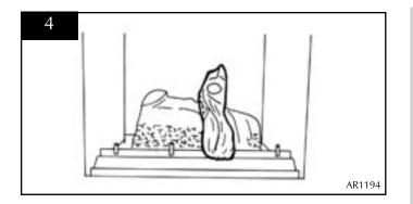
6.3 Place log C on the second stud and resting at the rear on log A. See diagram 5.
