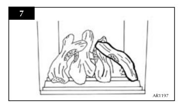
6.6 Place log F resting on the rear tray and leaning forward to locate in the recess in log E. See diagram 8.
