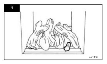
4.8 With the granules fill the front compartment around the logs evenly. ENSURE NO GRANULES FALL ON THE BURNER. See diagram 10.
