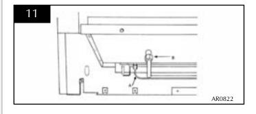
6.3 Remove the two screws retaining the valve bracket. See diagram 12.
