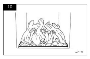
NOTE: ENSURE THAT THE LOGS ARE POSITIONED AS ABOVE. ONLY USE THE CORRECT AMOUNT OF LOGS AS SPECIFIED IN THE DIAGRAMS.
