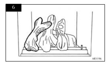
6.5 Place log E on to the last stud. The recess on the underside of the log should locate on to the top of log D. See diagram 7.
