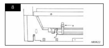
d) Remove the external feed pipe from the brass fitting. See diagram 8 arrow B.
