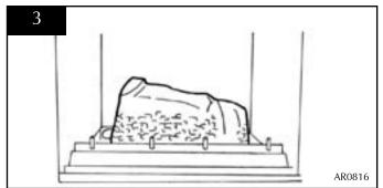
CENTRALISE THE LOG BETWEEN THE BURNERPORTS AT EITHER END.
