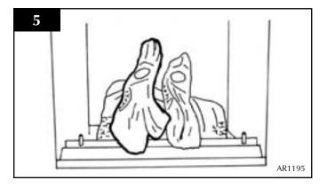
6.4 Place log B on the first stud. The recess on the underside of the log should locate on the top of log C. See diagram 6.
