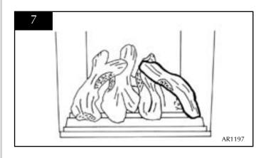
4.6 Place log F resting on the rear tray and leaning forward to locate in the recess in log E. See diagram 8.
