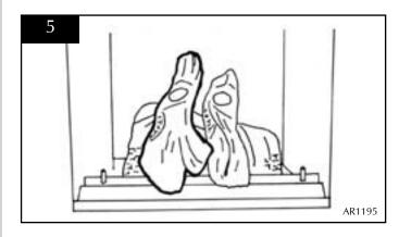
4.4 Place log B on the first stud. The recess on the underside of the log should locate on the top of log C. See diagram 6.
