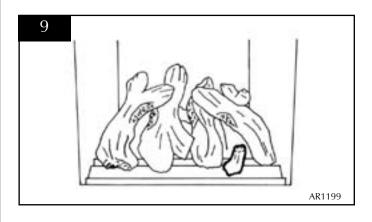
6.8 With the granules fill the front compartment around the logs evenly. ENSURE NO GRANULES FALL ON THE BURNER. See diagram 10.
