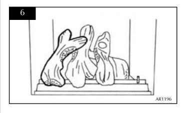
4.5 Place log E on to the last stud. The recess on the underside of the log should locate on to the top of log D. See diagram 7.
