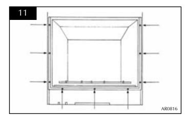
3.18 Carefully remove the box containing the logs and place to one side. Remove the cardboard fitment that protects the factory fitted ceramic panels; take care as these are easily damaged.
