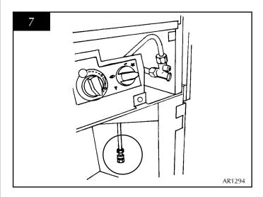
c) Disconnect the external pilot pipe from the brass fitting. See diagram 8, arrow A.
