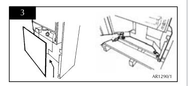
3.4 Gently remove the appliance from the crate and place into its intended position. Locate the two securing holes in the base subframe (those previously used to secure the appliance to the crate), mark the positions on the floor and place the appliance to one side. See diagram 4
