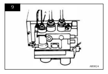
g) Push the thermocouple down through the hole in the base of the firebox and remove the component.
