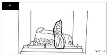
4.3 Place log C on the second stud and resting at the rear on log A. See diagram 5.
