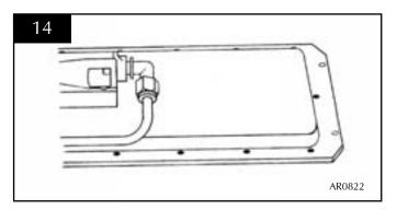
8.2 Rotate the injector until it is fully removed, and install the correct replacement injector. Re-assemble and turn the gas supply on, check for any leaks.
