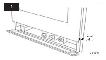
There are two fixing brackets either side of the controls:
