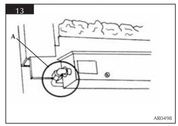
correct replacement injector. Reassemble and turn the gas supply on, check for leaks.
