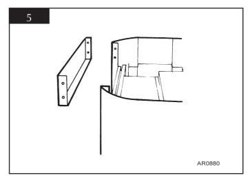
Locate the lower panels onto the lugs as shown. See diagram 6.
