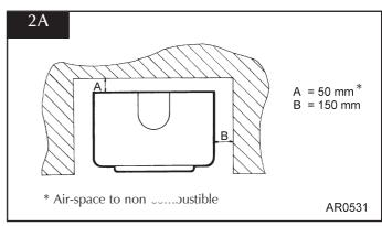
The above dimensions povide adequate clearance at the side and rear of the fire so that the controls can be reached.
