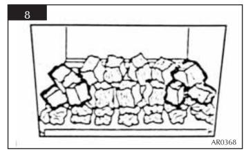
6.5 Place five small coals along the rear of the flame baffle, resting against the rear ledge, see diagram 9.
