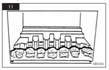
4.3 Place three large coals on the front coal so that they lean against the flame baffle, and the four large coals on the flame baffle so that they sit on the fingers, see diagram 12.
