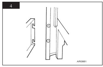
1.5 Lift the RH decorative panel to disengage from its locating brackets and remove from the stove, see diagram 4. It may not be necessary to remove the LH side.
