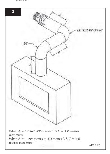
Any additional bend may be used on the horizontal section (either 45° or 90°), but the overall horizontal flue run will be reduced. Refer to Diagram 3.
