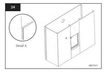
The top of the chimney breast must have a minimum  $200 \mathrm{cm}^2$  vent.
