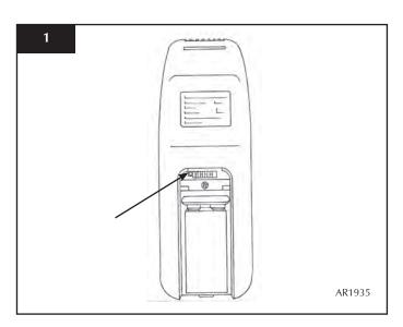
Each of the four switches can be set to either one of two positions, in any combination.
