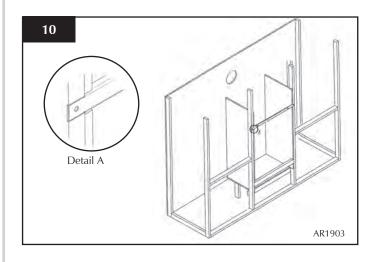
• Fit the support bar into the studwork at the correct height, Diagram 11.
