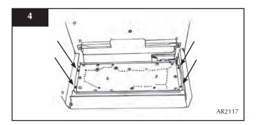
Undo the two screws in the rear air baffle to remove it,
