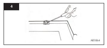
Lift the glass clear from the lock bracket at the top of the frame and slide out
