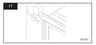
Build the studwork chimney breast to the desired size:
