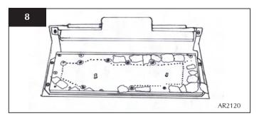
5.2 Place Log A onto the two studs on the burner skin, Diagram 9, with charred effect of the log facing forward.
