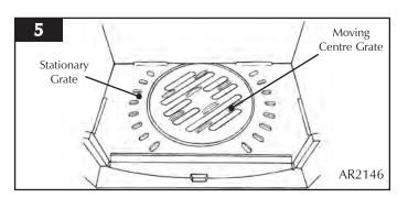
• Lift the moving grate parts, see picture 6
