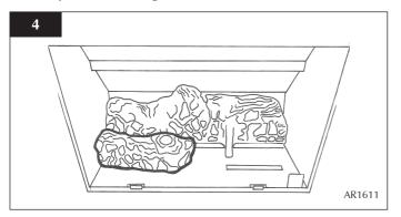
7.3 Place log C on the right-hand side of the burner with the location bar on the underside of the log fully located in the long slot in the burner. Make sure the log is as far right as possible. See diagram 5.
