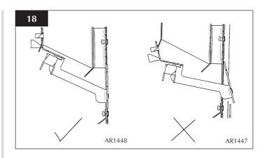
9.6 Feed the cable back through the hole as you replace the bracket. When the bracket is located correctly it will sit flush with the back panel without force required. If not positioned correctly the bracket will sit at an angle. See Diagram 18.
