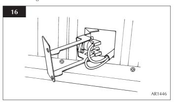
9.5 Refit the new sensor, ensuring that the plastic spacers are between the sensor and the bracket. Refit the leads. See Diagram 17.
