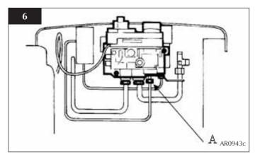
NOTE: Special care should be taken when replacing the thermocouple to the back of the gas valve ensuring that the sensor wires for the gazco flue sure system are not disconnected.
