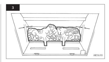
5.2 Place log B on the left-hand side of the burner with the location bar on the underside of the log fully located in the long slot of the burner. Make sure the log is as far to the left as possible. See diagram 4.
