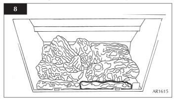
5.7 Place log E across from the rear of log A to log C on the right-hand side. Again, there are cut-outs for location. The front of the log should sit on the front ash panels and should fit tight to log C. See diagram 9.
