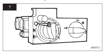
4.3 To release the right-hand side of the control cover insert the narrow blade screwdriver into the slot shown in diagram 8. Lever it gently and pull from the right-hand side at the same time. The cover will now come off. There is a small cylindrical metal spacer inside the cover; this must be kept and replaced on the fixing screw during reassembly.
