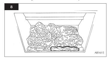
7.7 Place log E across from the rear of log A to log C on the right-hand side. Again, there are cut-outs for location. The front of the log should sit on the front ash panels and should fit tight to log C. See diagram 9.
