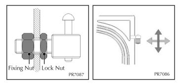
10.3 Using a 19mm A/F spanner loosen the fixing nuts, as shown, and reposition the hinge blocks to achieve a correct fit. This may require a trial and error approach to find the correct position.
