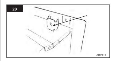
• Feed the wires for the remote touch pad through the grommet in the left side of the loose box
