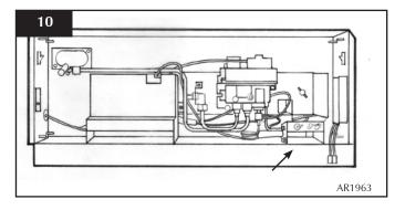
• Cut the cable tie retaining the vida flex sleeve and disconnect the ignition lead from the electrode
