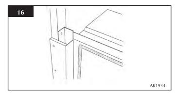
$\bullet\,$  Fix the edge of the vertical support flush to the edge of the channel
