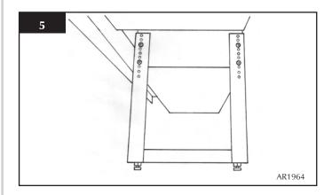
Build the stud work chimney breast and enclosures to the desired size to include the protected platform at the required height.
