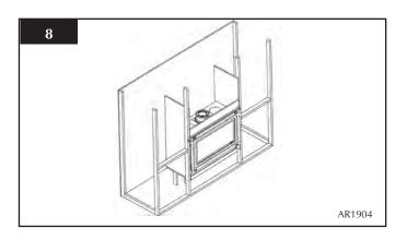
NOTE: If a frame is to be fitted, attach the brackets before installing the appliance.
