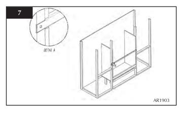
• Fit the supplied top support bar into the stud work at the correct height, Diagram 8, because no combustible material can be used above the fire
