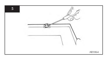
• Lift the glass clear from the lock bracket at the top of the frame and slide out
