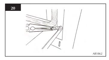
• Raise the door to almost upright and move the door left This releases the left-hand side off its hinge pin
