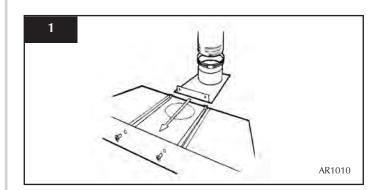
When installing the appliance into a masonry chimney without a liner, it must be converted to a rear exit:
