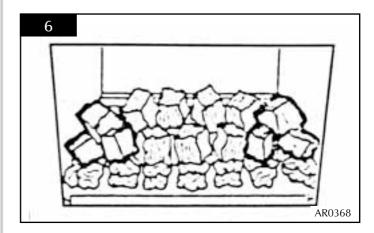
6.5 Place five small coals along the rear of the flame baffle, resting against the rear ledge, see diagram 7.
