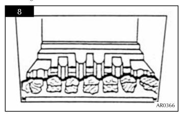
3.11 Place three large coals on the front coal so that they lean against the flame baffle, and the four large coals on the flame baffle so that they sit on the fingers, see diagram 9.
