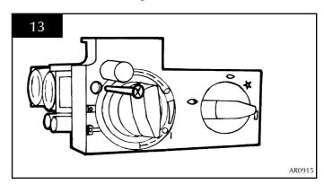
To release the right-hand side of the control cover, insert the narrow blade screwdriver into the slot shown in diagram 11. Lever it gently and pull from the right-hand side at the same time. The cover will now come off. There is a small cylindrical metal spacer inside the cover. This must be kept and replaced on the fixing screw during re-assembly.
