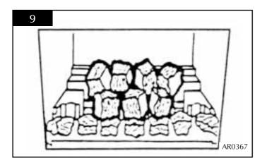
3.12 Place two small coals at each end of the front coal so that they lean against the flame baffle, and a further two large coals on the flame baffle, one at each end, see diagram 10
