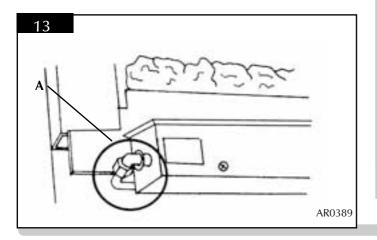
8.2 Rotate the injector until it is fully removed, and install the correct replacement injector. Reassemble and turn the gas supply on, check for leaks.
