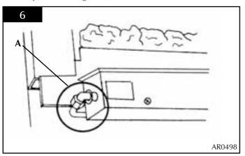
2.4 Remove the 2 screws attaching burner to back of unit, see diagrams 7. Carefully withdraw burner unit upwards and tilt to remove the burner through door opening. Remove the 2 screws holding the heat shield in place.
