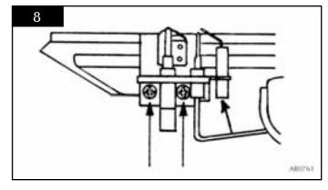
3.2 When replacing the pilot ensure the thermocouple follows its original route, i.e. along the pilot pipe. Attach the thermocouple to the pipe with new cable ties.
