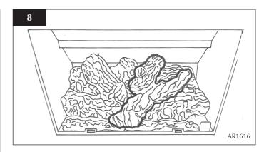
7.8 Carefully insert the front coal retainer into the front panel of the firebox. Take care not the scrape/damage the logs. This coal retainer sits in two brackets. Ensure it is fully inserted, leaving approximately a 4 mm gap between the firebox ledge and the bottom of the coal retainer.
