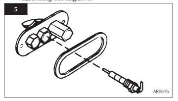
3.6 To remove the thermocouple, undo the retaining nut and withdraw the thermocouple, see diagram 6. Undo the thermocouple from the back of the gas valve, see diagram 7, arrow A. Reassemble in reverse order. Do not overtighten.
