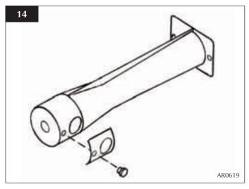
9.5 Reassemble in reverse order with correct aeration plate(s). NOTE: EVEN IF NO AERATION PLATE IS REQUIRED, THE SMALL SCREW(S) MUST BE REPLACED.
