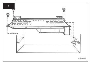
2.3 To replace the burner, engage the venturi over the injector ensuring the burner sits on top of the fixing bracket. Push the burner to the right and whilst holding, insert the three fixing screws.
