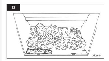
5.4 Place the second ash panel to the right of the first, with the pointed end of the panel fitting into the V shape. This panel should locate on the screw holes of the burner skin. Ensure that both logs are horizontal to the burner ports.
