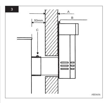
Any terminal which is less than 2 meters above any access (level ground, balcony or above a flat roof to which people have access), is to be fitted with the guard supplied, see diagram 4.
