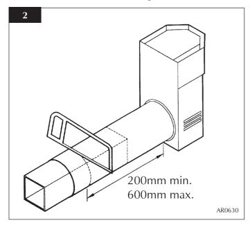
3.1.6 From outside, locate the flue assembly into the hole until the terminal is flat against the wall. Ensure the terminal is vertical. NOTE THE ORIENTATION OF THE TERMINAL. See diagram 3. Mark the four fixing holes, remove the terminal and drill the holes, inserting the rawplugs supplied.
