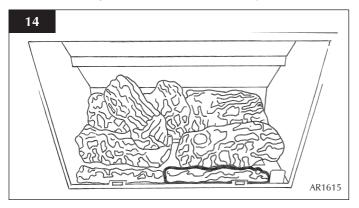
5.5 Place log E across from the rear of log A to log C on the right hand side. Again, there are cut-outs for location. The front of the log should sit on the front ash panels and should fit tight to log C. See diagram 15.
