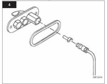
3.5 To remove the electrode, disconnect the ignition lead and undo the retaining nut. The electrode can now be removed, note the orientation of the electrode terminal when reassembling. See diagram 5.
