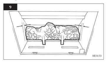
5.8 Place log B on the left hand side of the burner with the location bar on the underside of the log fully located in the long slot of the burner. Make sure the log is as far to the left as possible. See diagram 10.
