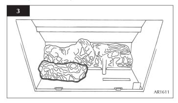
7.3 Place log C on the right hand side of the burner with the location bar on the underside of the log fully located in the long slot in the burner. Make sure the log is as far right as possible. See diagram 4.
