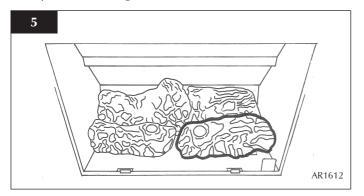
7.4 Place log D across from the rear log A to log B on the left-hand side. There are cut-outs in both logs for location. See diagram 6.
