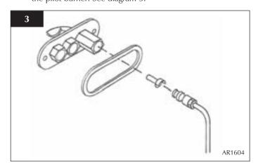
3.6 To remove the electrode, disconnect the ignition lead and undo the retaining nut. The electrode can now be removed. Note the orientation of the electrode terminal when reassembling. See diagram 4.
