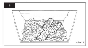
7.8 Carefully insert the front coal retainer into the front panel of the firebox. Take care not the scrape/damage the logs. This coal retainer sits in two brackets. Ensure it is fully inserted, leaving approximately a 4 mm gap between the firebox ledge and the bottom of the coal retainer.
