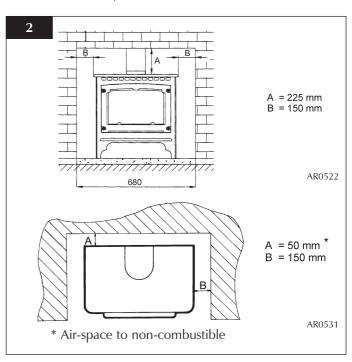
The above dimensions provide adquate clearance at the side and rear of the fire so that the controls can be reached.
