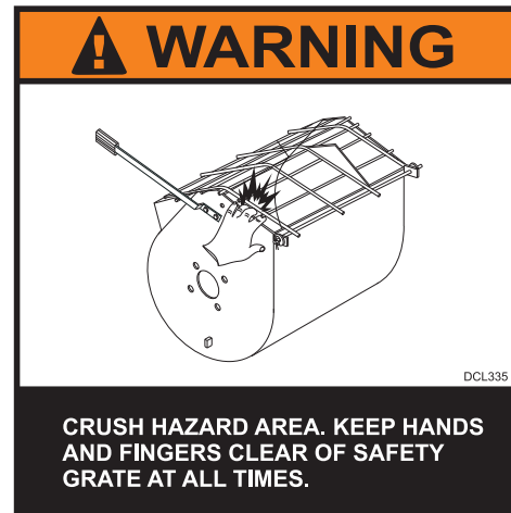
Figure 37. Safety Grate (Crush Hazard)
