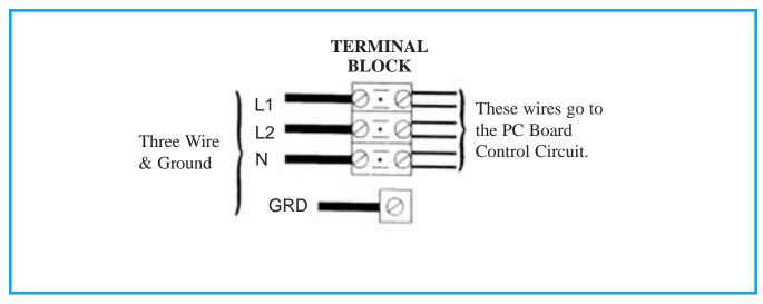
Connections should be made using copper conductors only. The connecting wire and circuit breakers or fuses must be sized to accommodate the total ampere load as specified on the equipment module data label.
