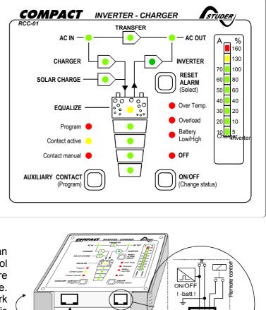
The Control Input is connected in parallel to the ON/OFF- push button. The COMPACT can be switched on or off through this input with an impulse button or an impulse contact.
