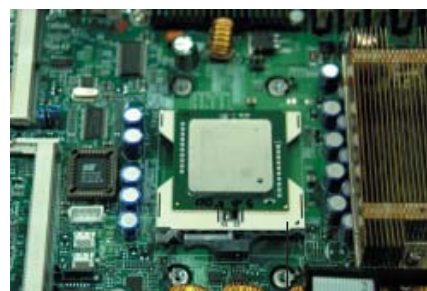
Socket lever in the locking Position
