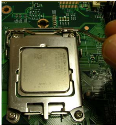
Figure 2-5. Secure the CPU with Socket Lever
