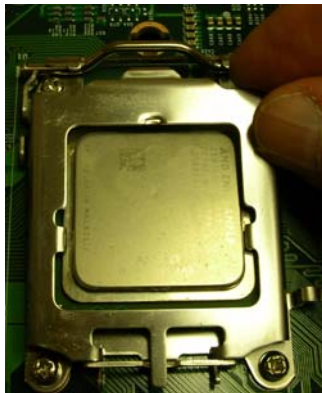
Figure 2-4. Inspecting the CPU Installation
