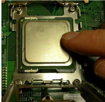
Figure 2-3. Placing the CPU into the Socket
