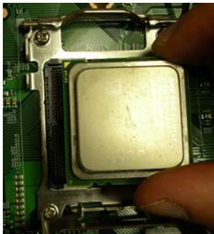
Figure 2-2. Aligning the CPU with Socket
