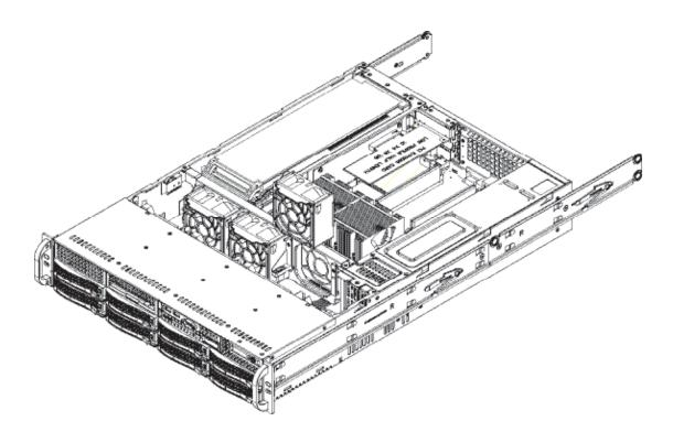
Figure 6-2. Removing System Cooling Fans
