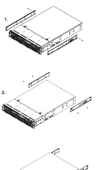
Figure 2-1. Installing Chassis Rails
