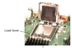
CPU installed in socket
