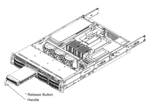
Figure 6-4. Removing a SAS/SATA Drive Carrier
