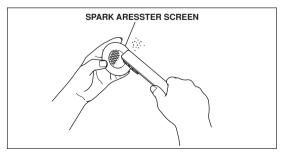
Install the spark arrester, and muffler protector in the reverse order of disassembly.
