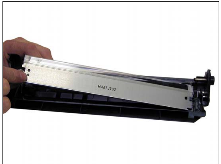
13. Remove the wiper blade from the cartridge and clean out the waste toner.
